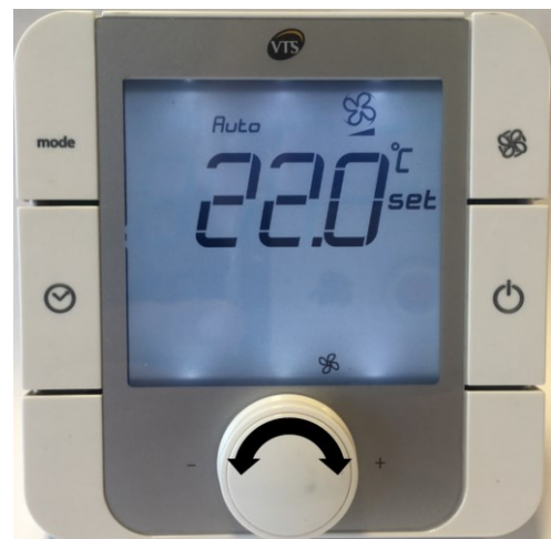
Figure 37 - HMI Basic. Temperature set-point
